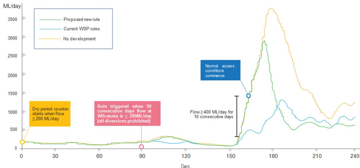
**Figure 2: Example of flow with the resumption of flow rule at Wilcannia**
