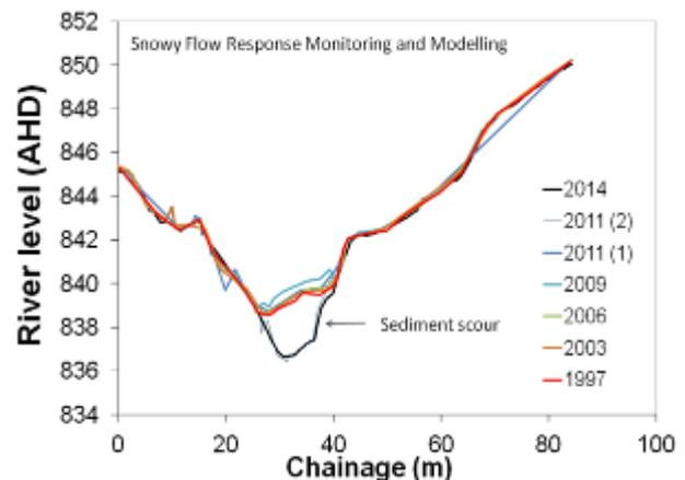
**Figure 6. Localised change in channel morphology in the Snowy River downstream of the Mowamba River (Site 1- cross section 6) following the introduction of high flows in 2011** (source: S. Williams).
