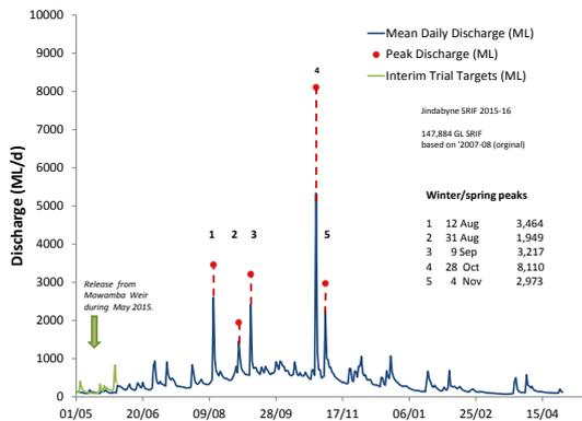
**Figure 2. Snowy River below Jindabyne mean daily discharge pattern for 2015-16 (blue), with one primary (4) and four secondary (1,2,3,5) 8-hourly flow peaks (red dotted lines).**
