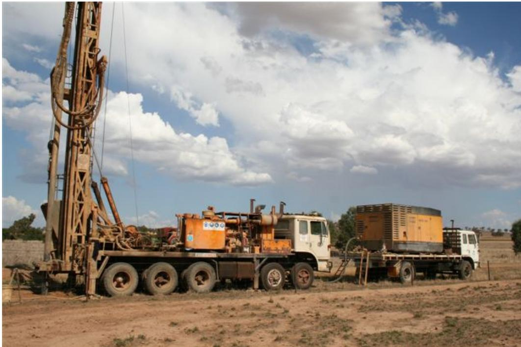
**Figure 2-2 Air Rotary Drill Rig**
