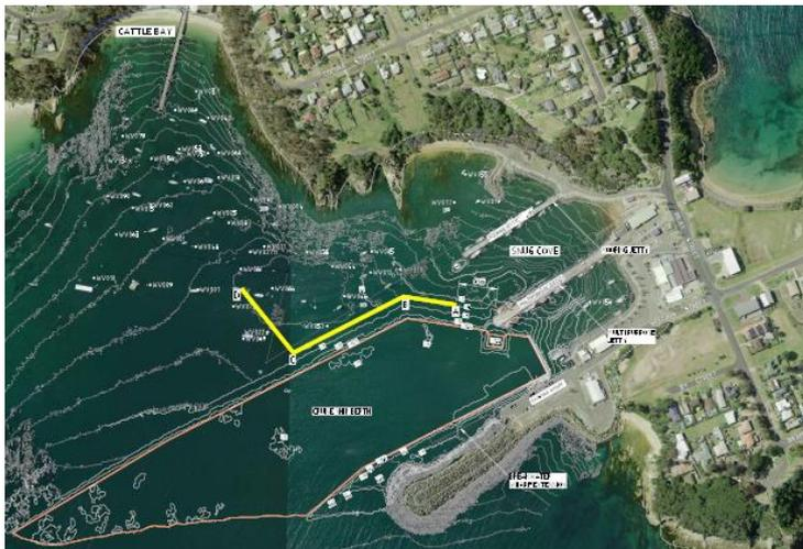
Final wave attenuator alignment
