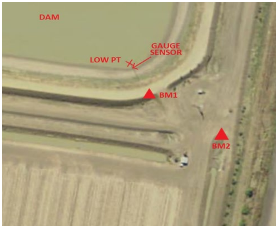
Figure 3. Close up aerial image of storage with survey information.
