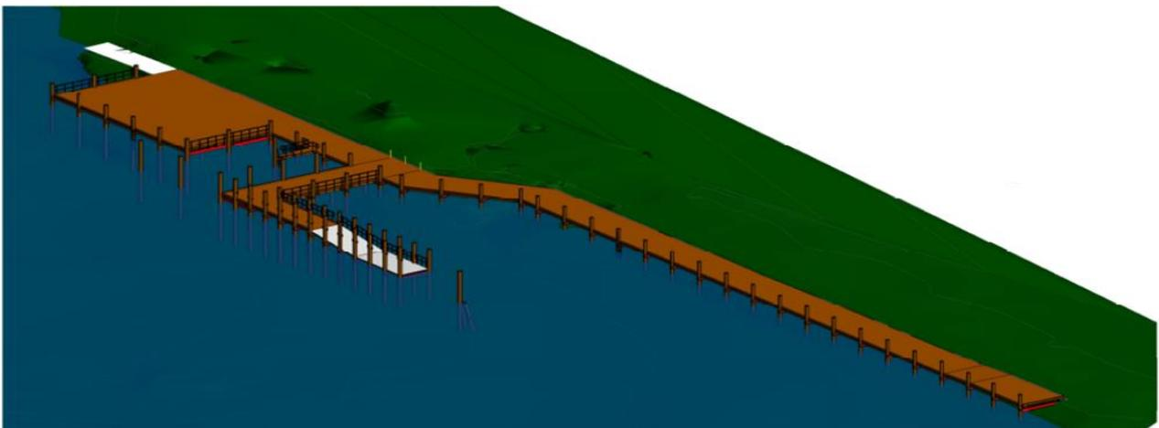
**Figure 1. Design drawing of the jetty and boardwalk structure**
