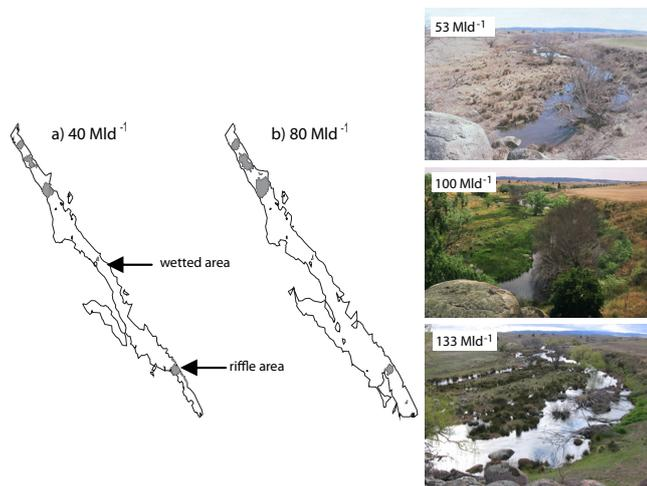
Figure 1 (left): HEC-GeoRAS hydraulic model of Snowy River at Blackburn Creek showing a 50 per cent increase in total wetted area and riffle area at river flows from a) 40 Mld<sup>-1</sup> (mega litres per day) and b) 80 Mld<sup>-1</sup>. Photo-point monitoring of the Snowy River at 53, 100 and 133 Mld<sup>-1</sup>.
