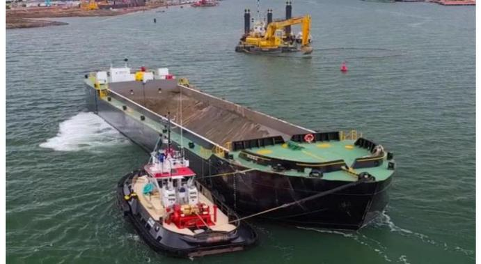
**A typical split hopper barge assisted by a tug boat**
